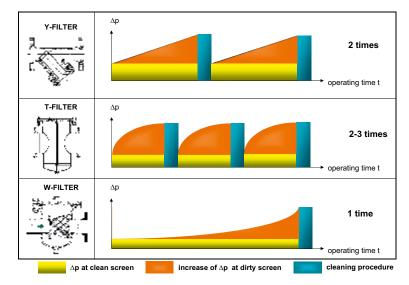
Figure 6: Cleaning intervals of different types of strainers
