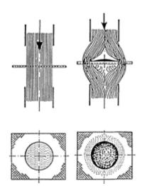
**Figure 3:** Flow path in a T-Filter under clean (left) and dirty conditions (right)
